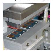
unit production. The temperature resistance in the application requires a high glass-transition temperature of the adhesive, which drives up the heatseal temperature. The polyimide adhesive on our TPI bond film is be heatsealed at 250-300°C. A diagram of a PowerFlex printed circuit (based on TPI bond film) appears below:
