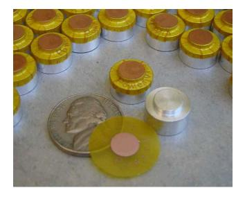
PowerVias are inserted in the 'underside' of a FR4 printed circuit board (the power components would be soldered to the 'topside'). The fully-assembled PCB is not attached to the heat sink, with thermal grease or phase-change material under the PowerVia columns.
